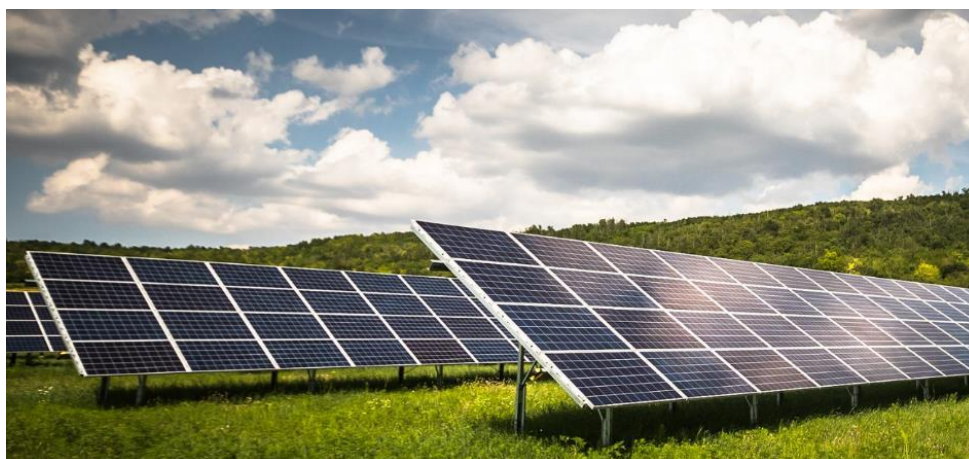
Figure 5-7: Fixed tilt system 5
